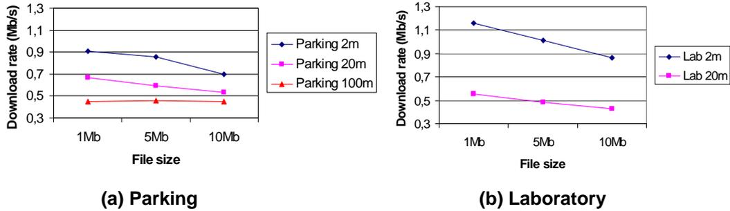
Figure 3: Average download rates considering different distances and file sizes in the Parking(a) and Laboratory(b) scenarios
