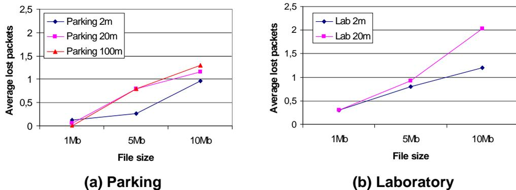
Figure 4: Average of lost packets considering different distances between the devices and file sizes in the Parking(a) and Laboratory(b) scenarios
