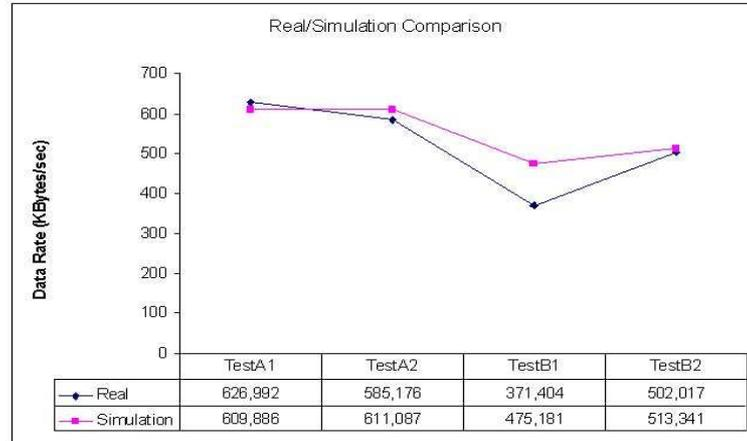
Figure 9: Comparison between real and simulation transmission rates
